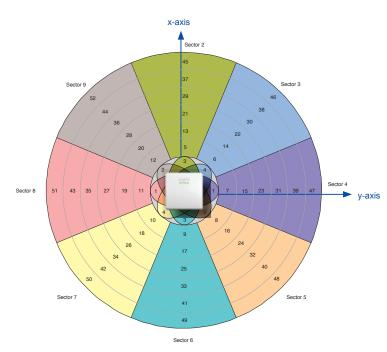
The Speedway xArray reader system can distinguish 52 different antenna beams providing location assignment and wide —area monitoring.
